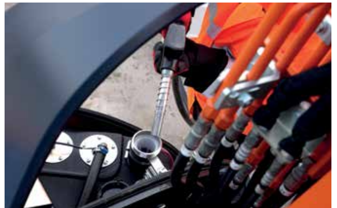
The fuel tank has also been repositioned to make it easier and safer to refill.
