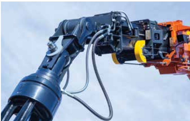
Rotation piping included for swivel clamshell buckets (ZX350-7 30m CTA).
