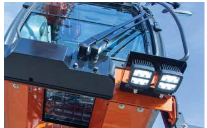
LED lights highlight the working area for operators.
