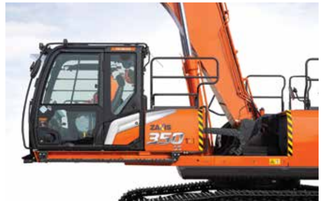
The sliding cab enhances visibility and safety.
