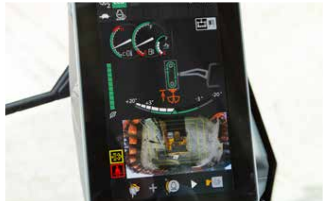
Standard screen includes telescopic indicator display.
